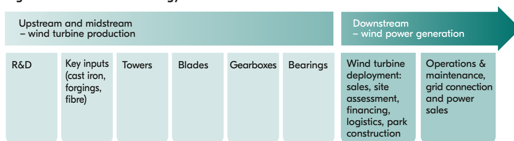
Figure 3. Onshore wind-energy value chain
